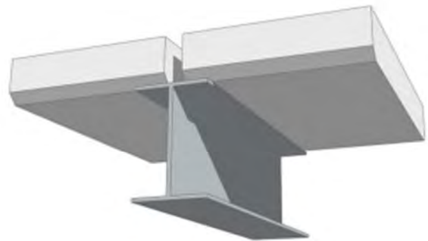
Sub-standard bearing on 100mm beam
