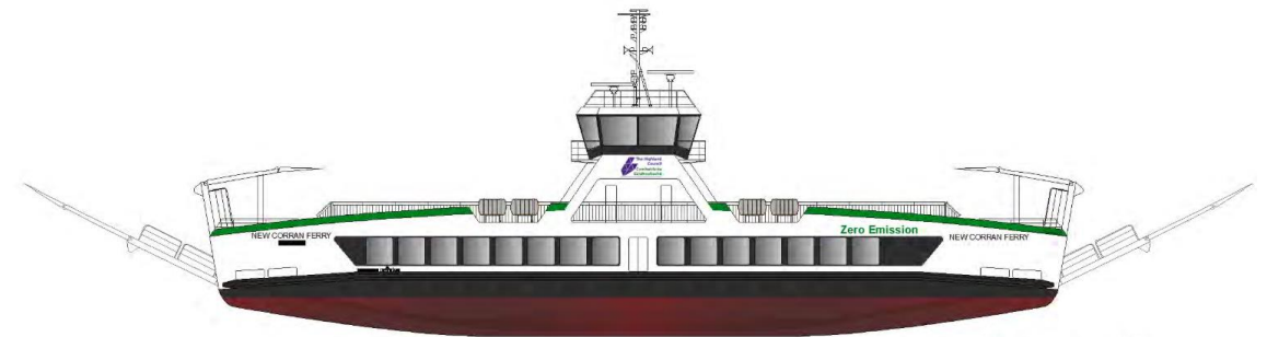
New Corran Ferry - All Electric 32 car
