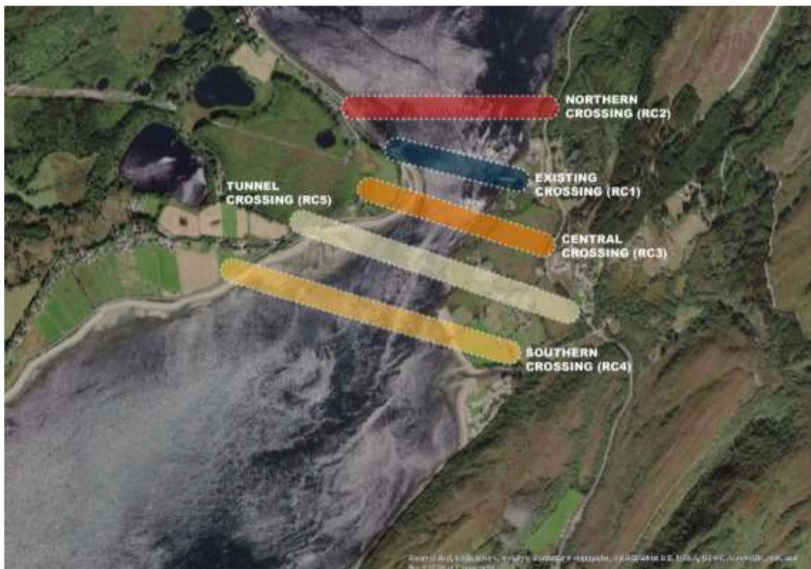
Figure 3-1: Corran Narrows Route Corridors (Stantec, 2019)
