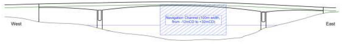
Figure 3-9: Box girder bridge with conventional piers
