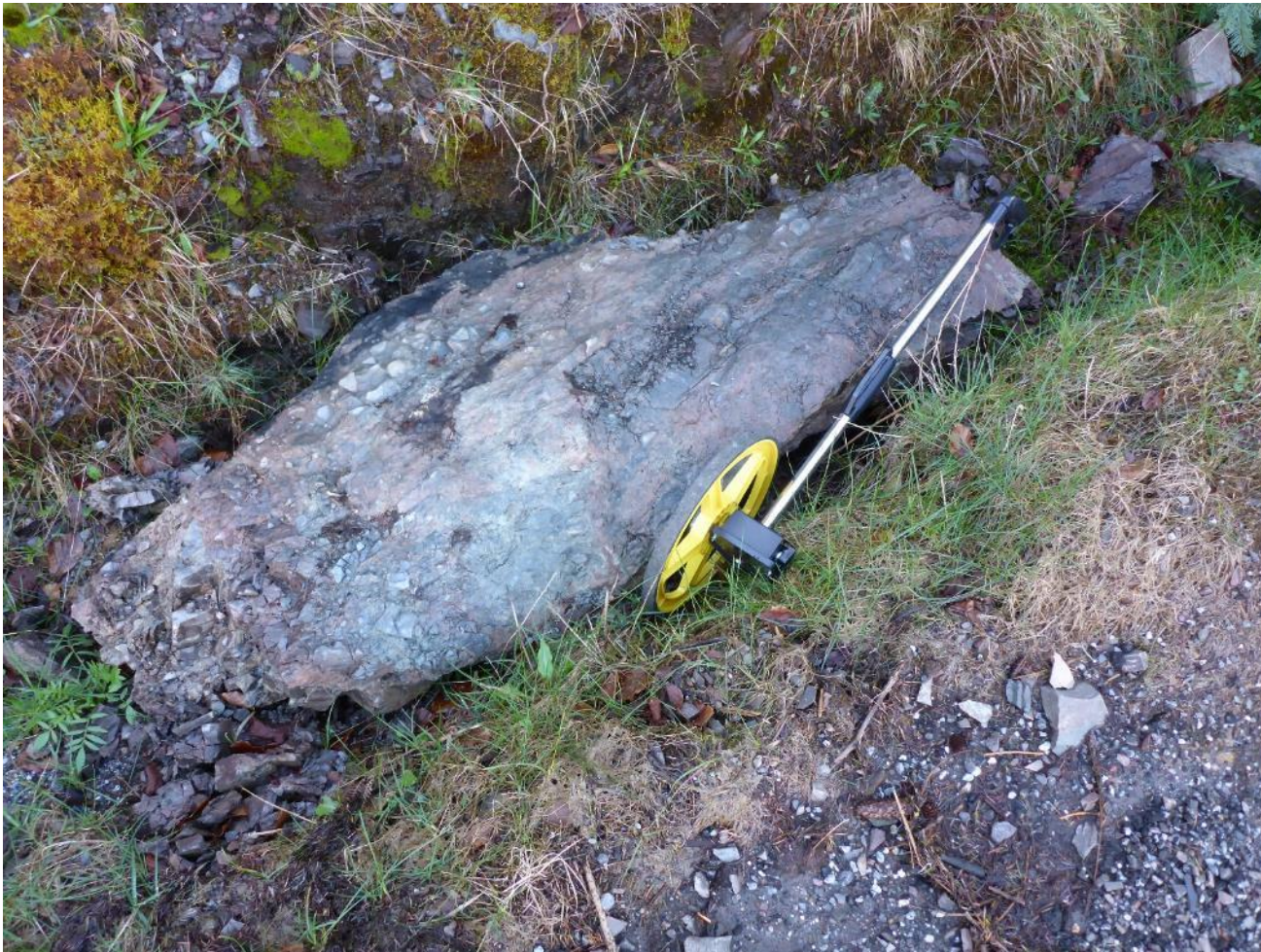
Ch. 31 – Large block (1.0m x 0.5m x 0.4m) in ditch.
