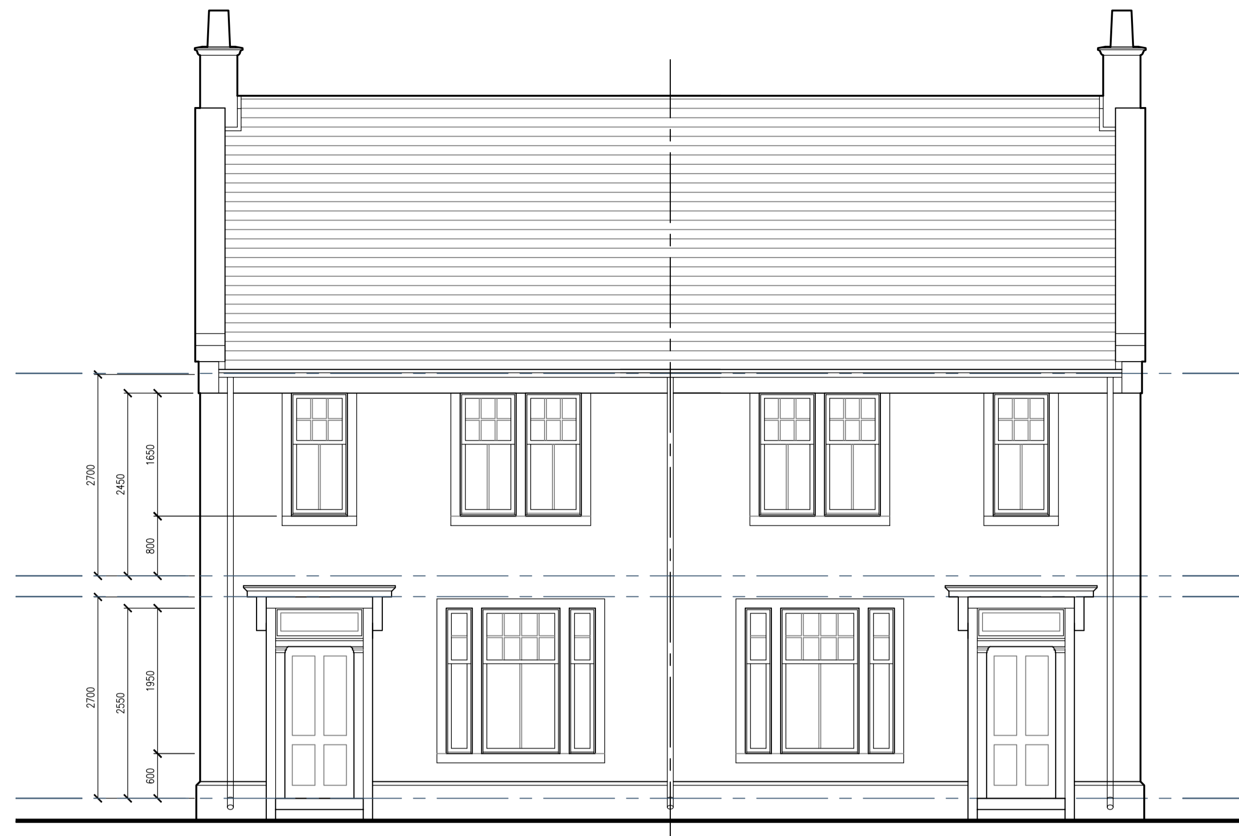
3 FRONT ELEVATION: VICTORIAN (SEMI-DETACHED CONFIGURATION) H5.2 SCALE = 1:50
