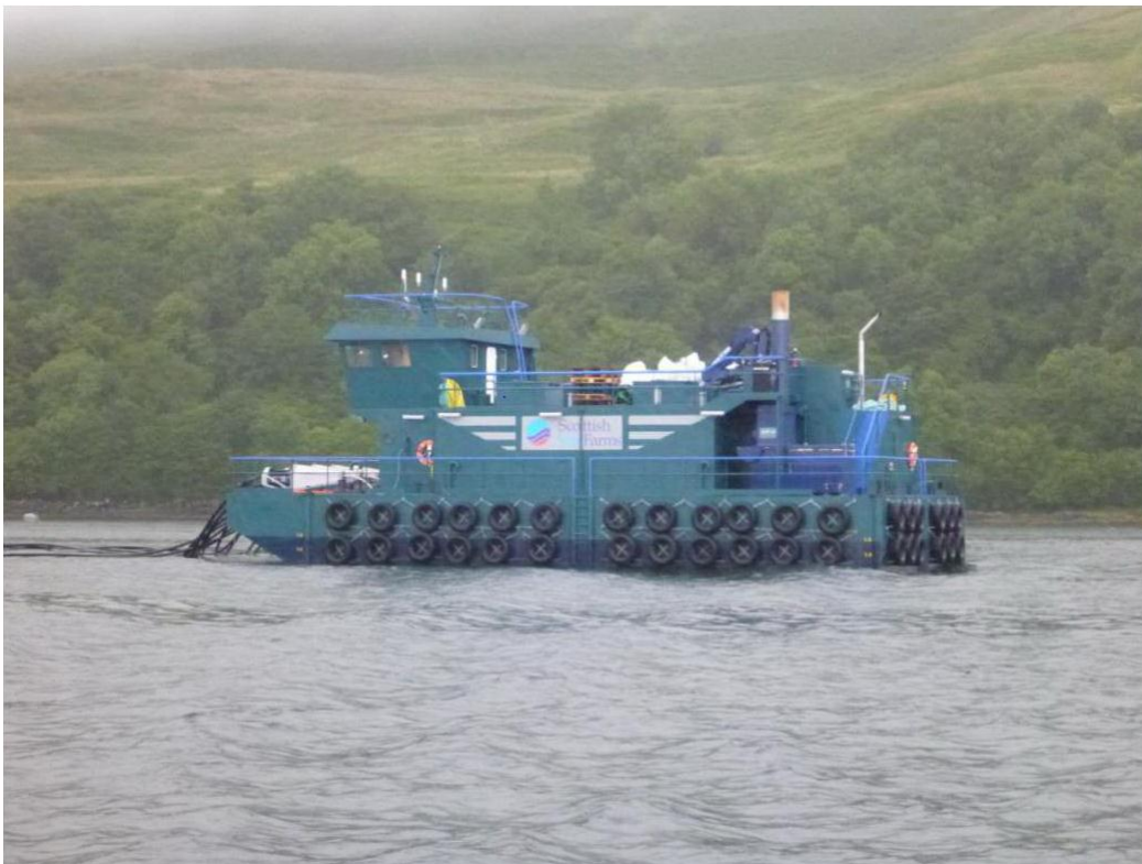
Diagram 4: Example of proposed Macduff feed barge (170 tonnes capacity)
