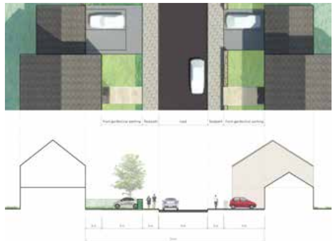
FIGURE 28 Section - Northerly Primary Street
