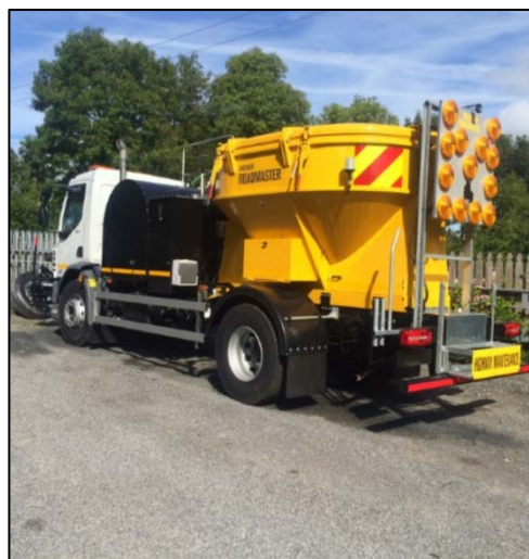
Figure 3.1.2: Spray Injection Repair Vehicle
