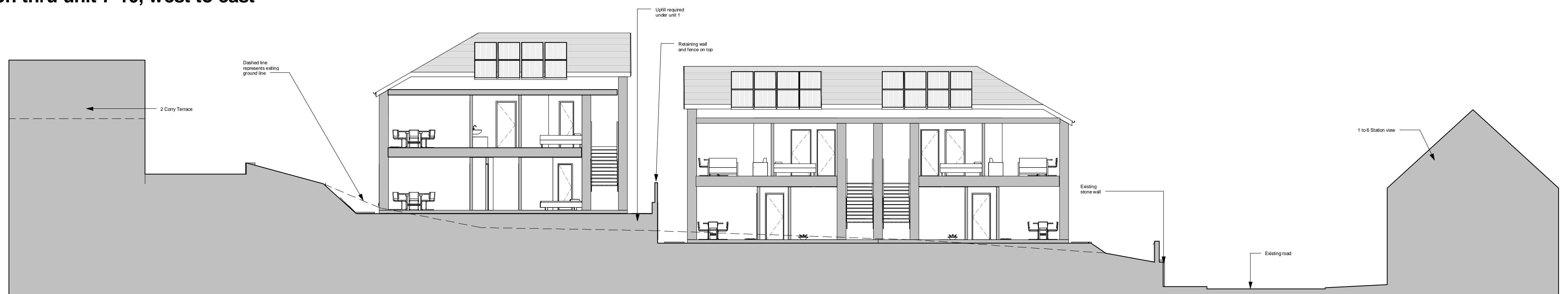
Section thru units 1-6, west to east
