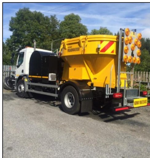
Figure 3.1.2: Spray Injection Repair Vehicle
