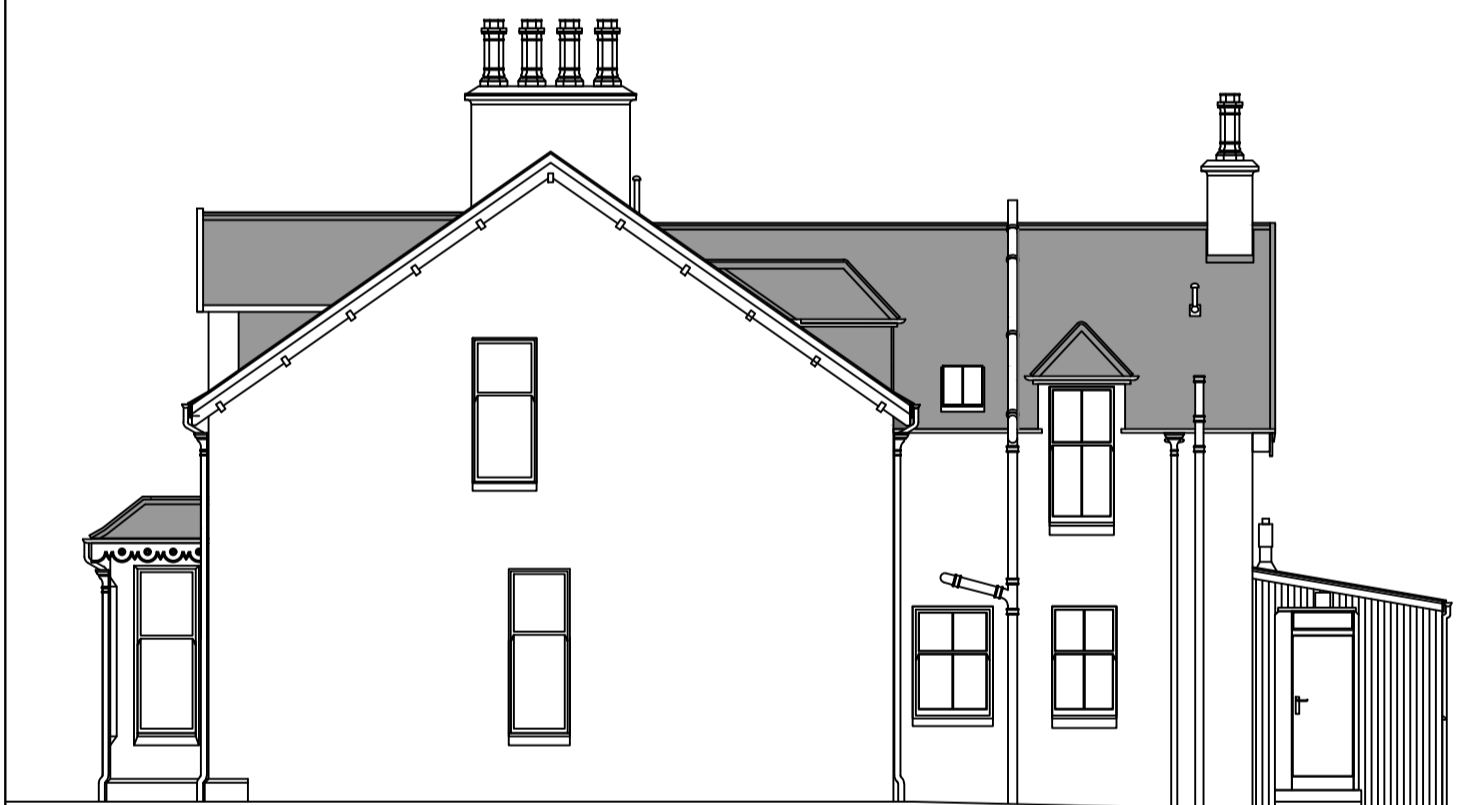
East Elevation - Existing
