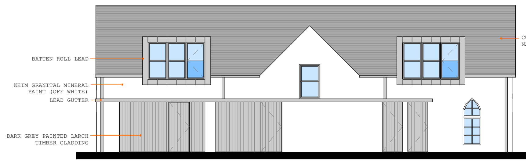
Proposed NE Elevation - 1:100
