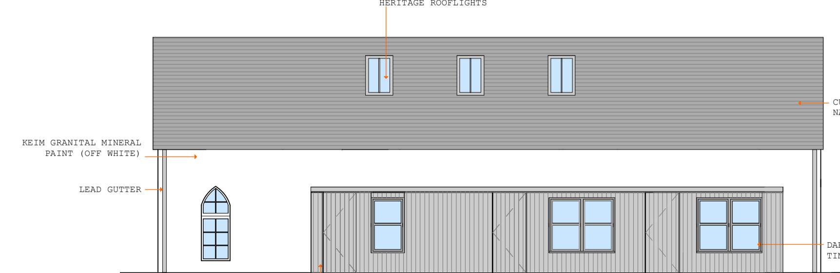
Proposed SW Elevation - 1:100
