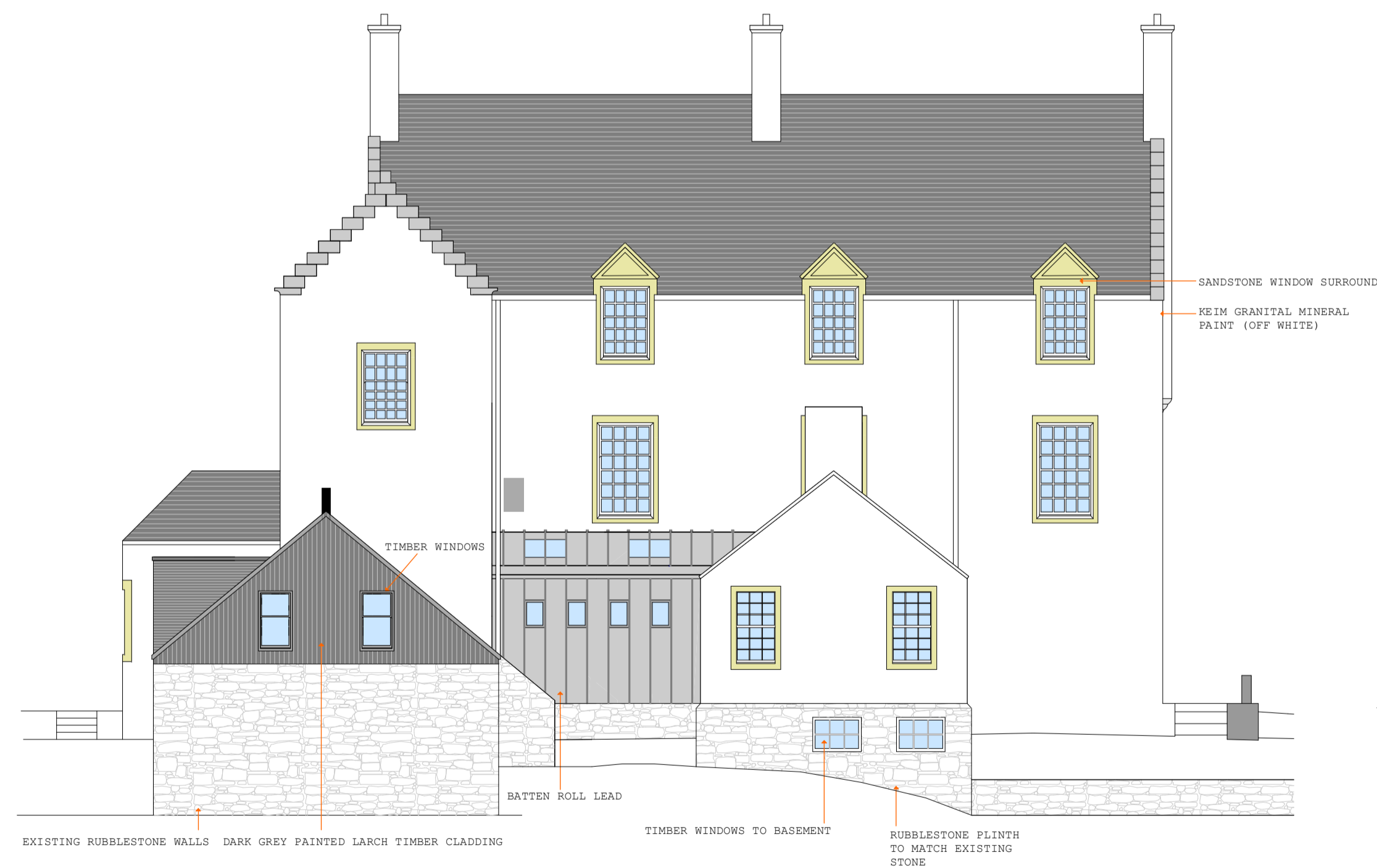
Proposed Elevation C - 1:100
