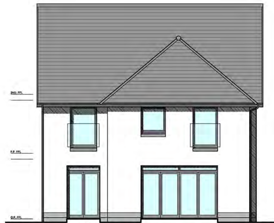
REAR ELEVATION (WEST) [Handed to units 10 & 11]
