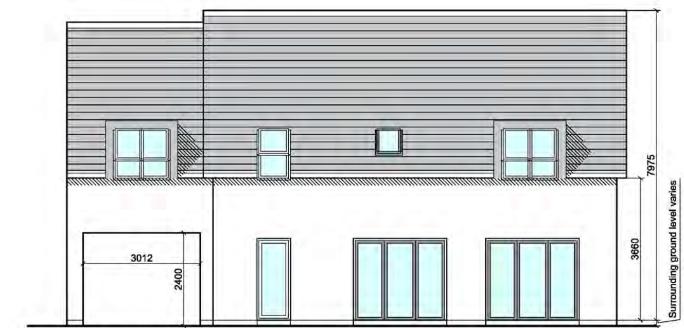
REAR ELEVATION (EAST) [handed to unit 37]
