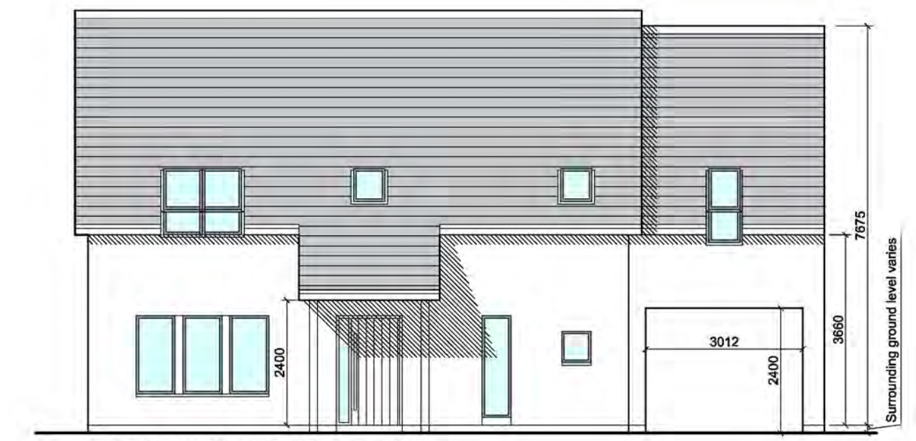
FRONT ELEVATION (WEST) [handed to unit 37]
