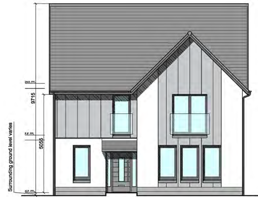
FRONT ELEVATION (EAST) [Handed to units 10 & 11]
