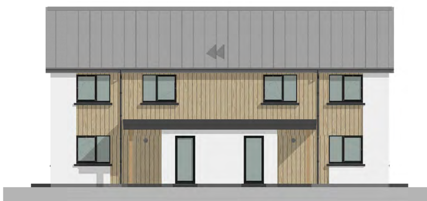
Front (Entrance) Elevation Scale - 1 : 100
