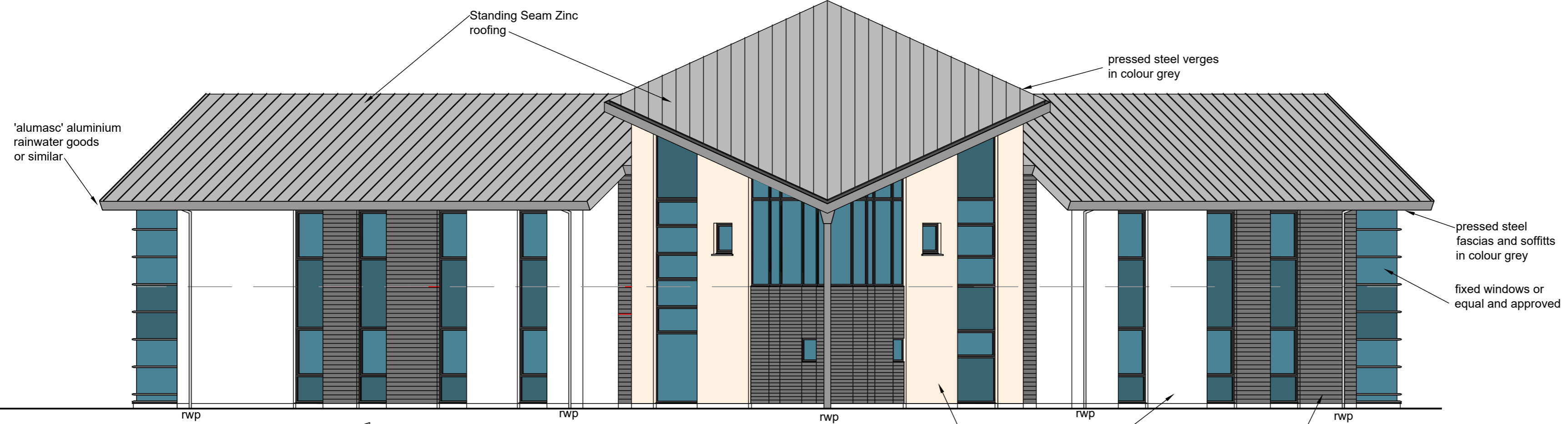
North and East Facing Elevations 1:100
