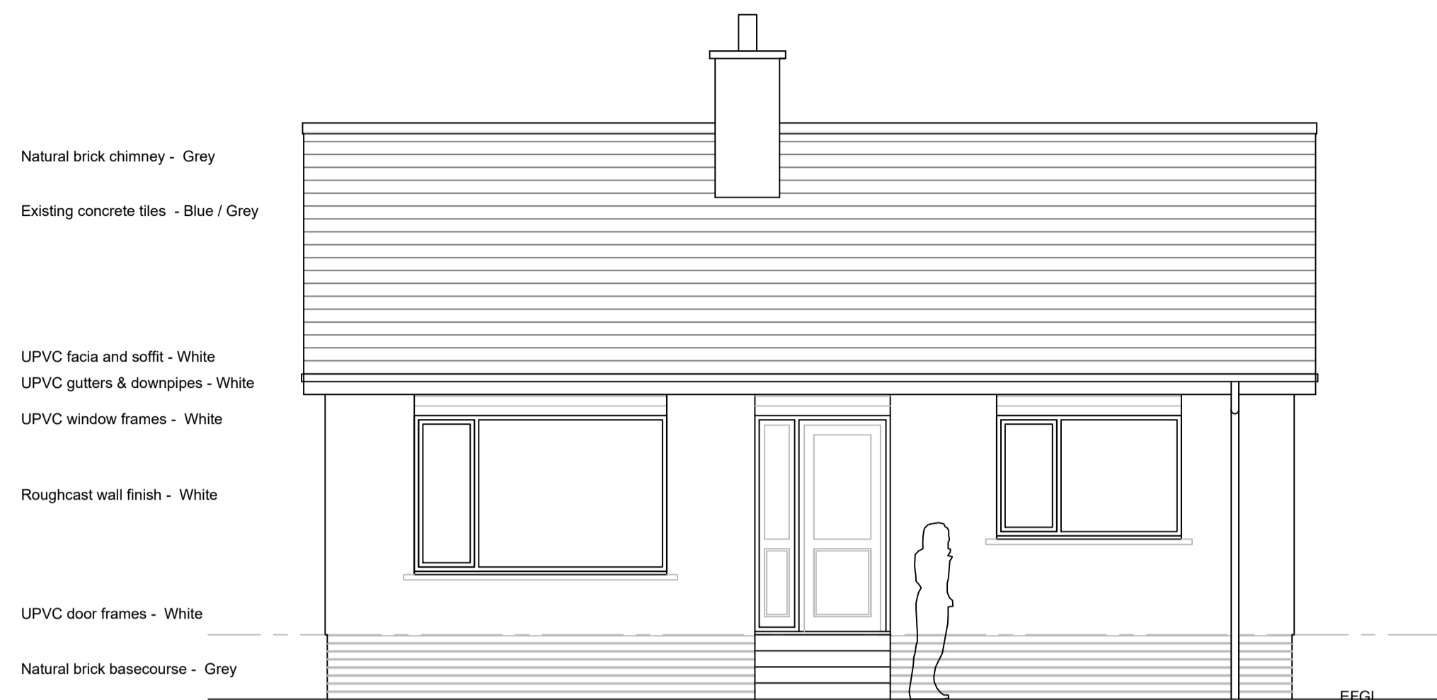
Front (South) Elevation 1:100
