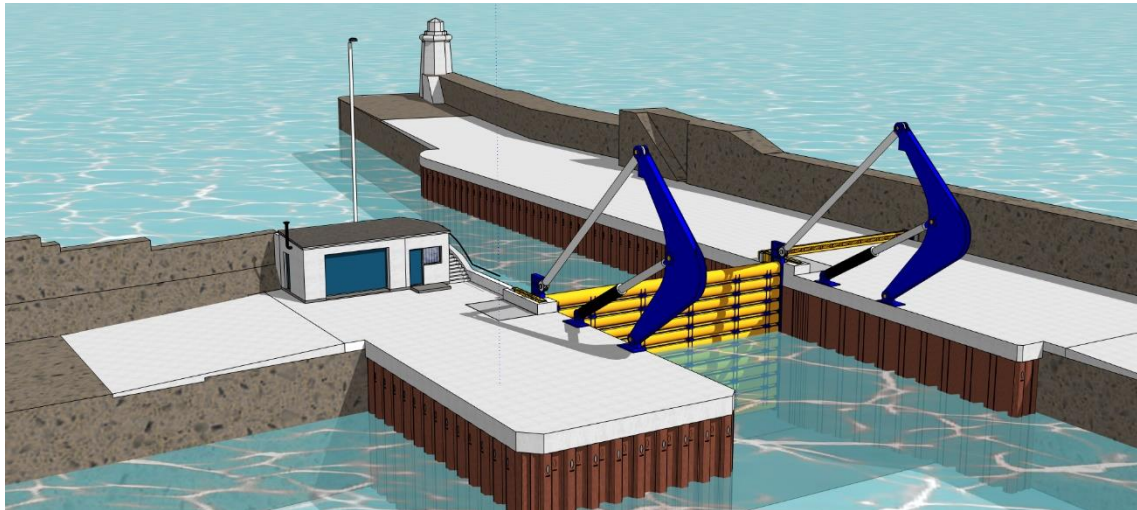
The proposed High Water Protection Gate
