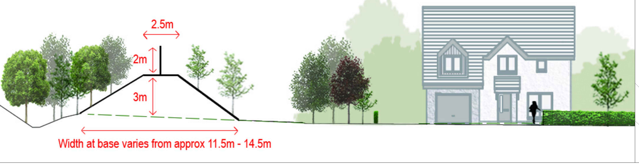
Section A-A through Acoustic Bund and Plot 77
