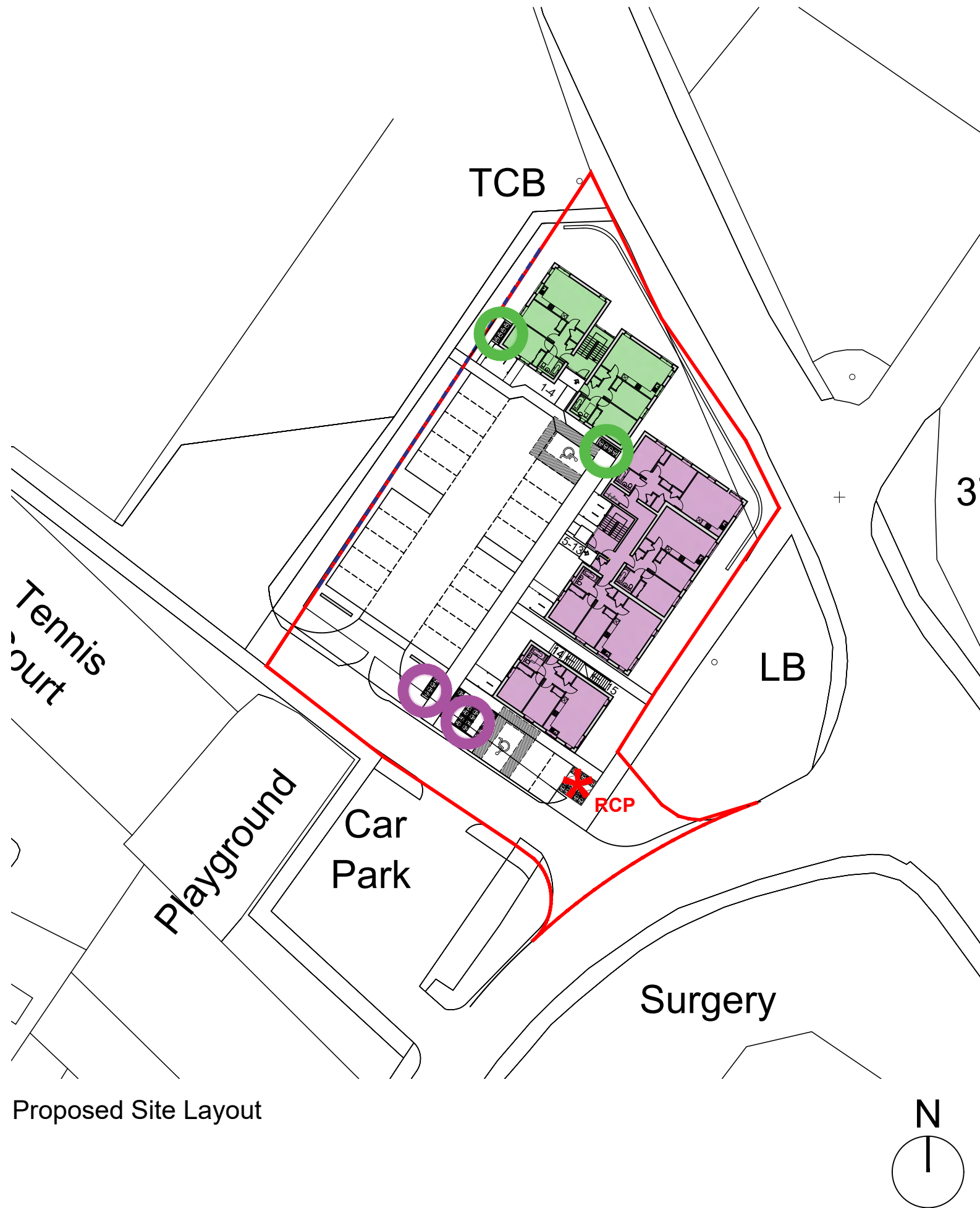
Main Bin Store Area (capacity for storage of 22 no. 140 litre waste bins)
