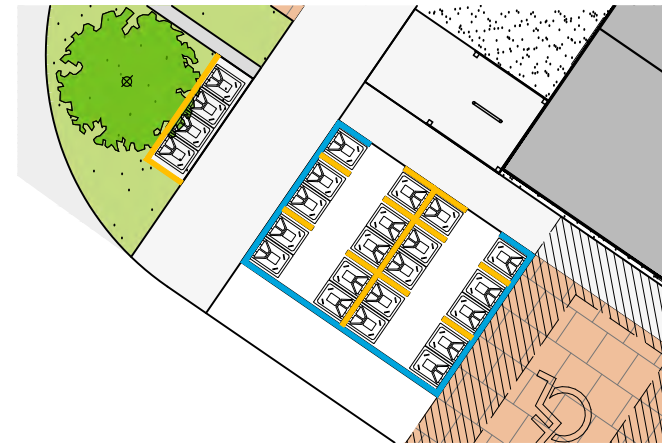
Main Bin Store Area (capacity for storage of 22 no. 140 litre waste bins)
