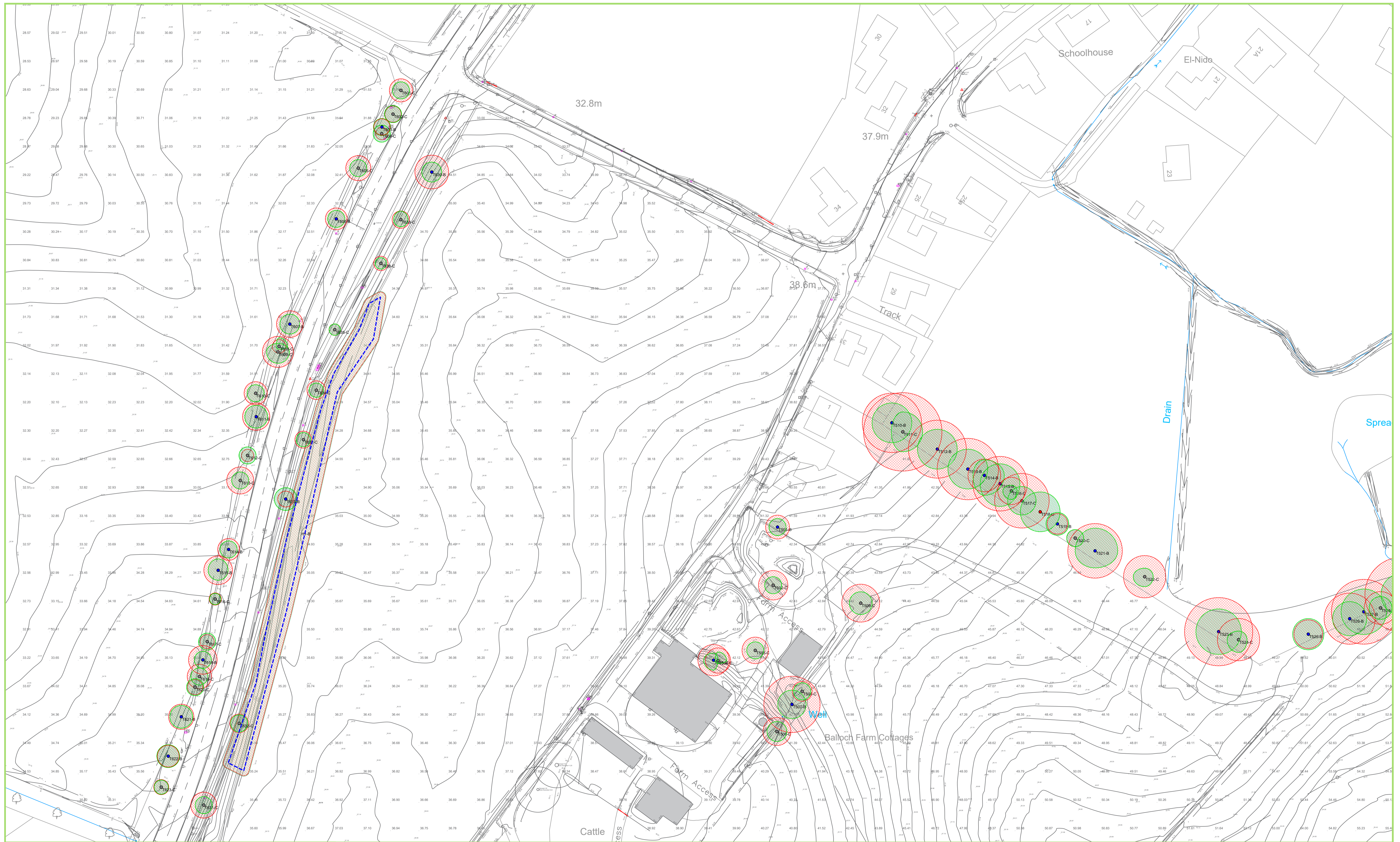
Tree Constraints Plan showing tree categories and root protection zones. BS5837:2012 Tree Categories
