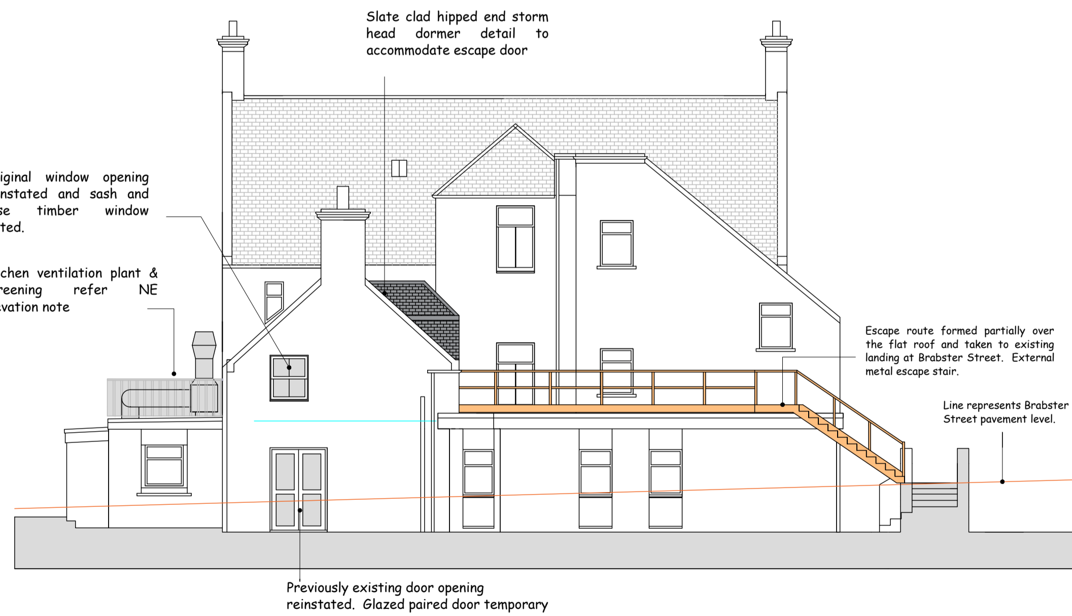
NORTH WEST ELEVATION WITHIN SITE
