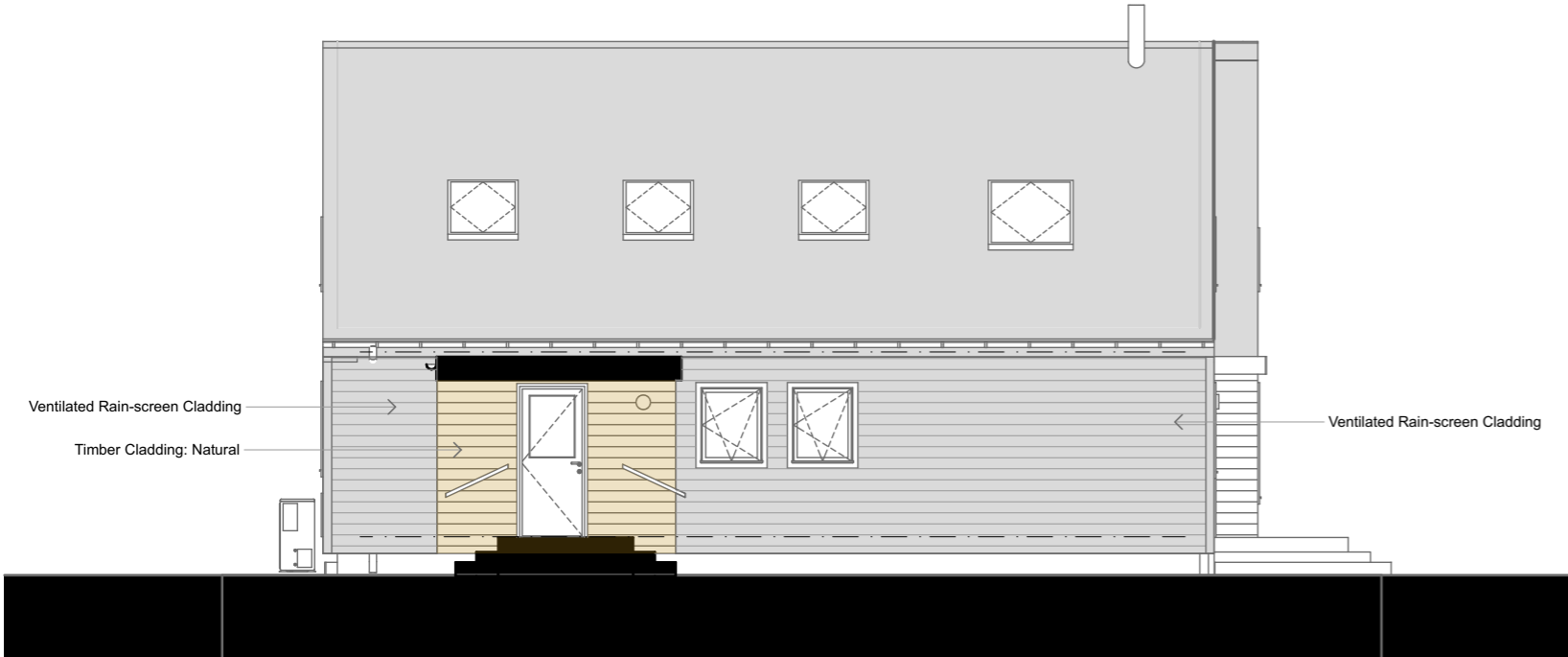
1:100 North West (Drive) Elevation NW1
