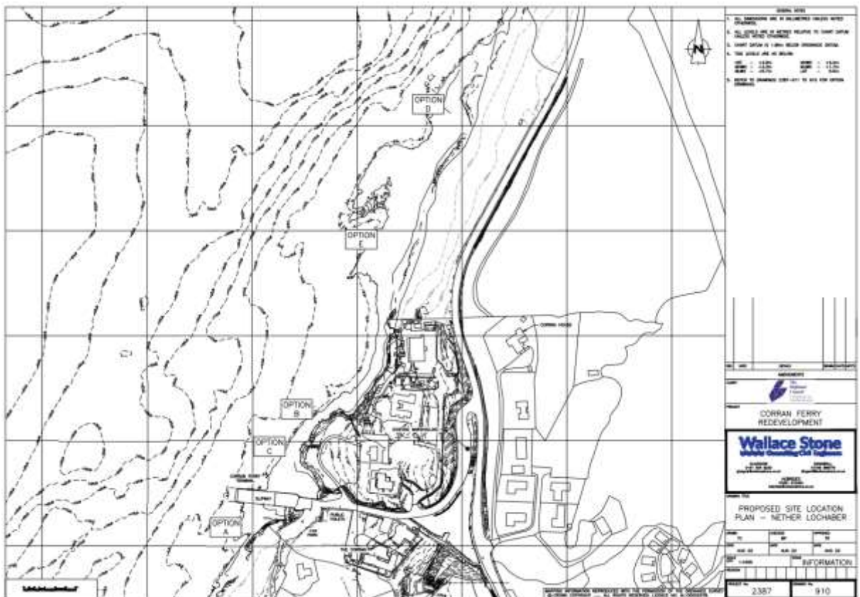
Figure 4.2: Corran / Nether Lochaber infrastructure options
