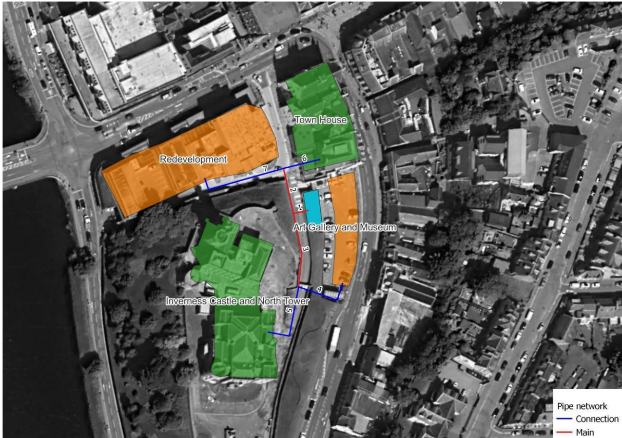
Figure 8.3: Buried network for the Castle area
