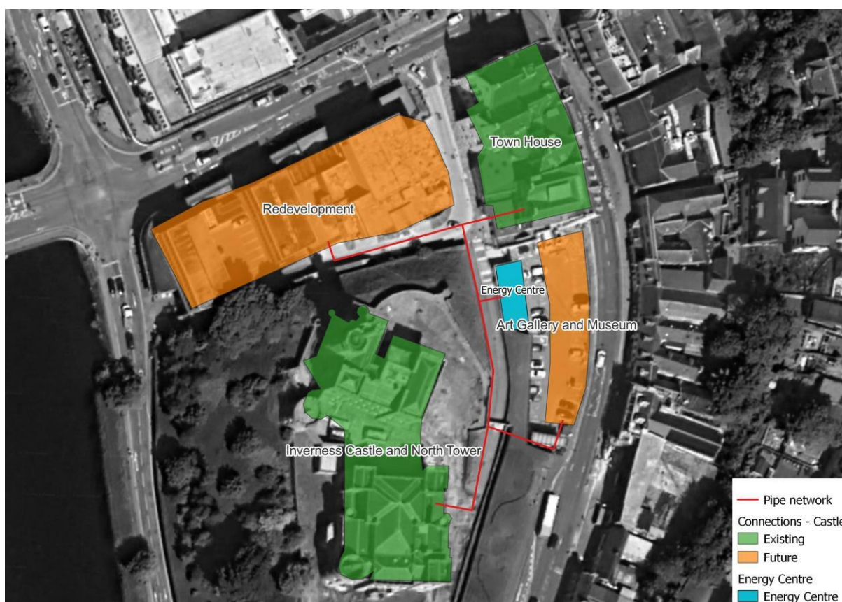
Figure 8.1: Indicative Buried Network route
