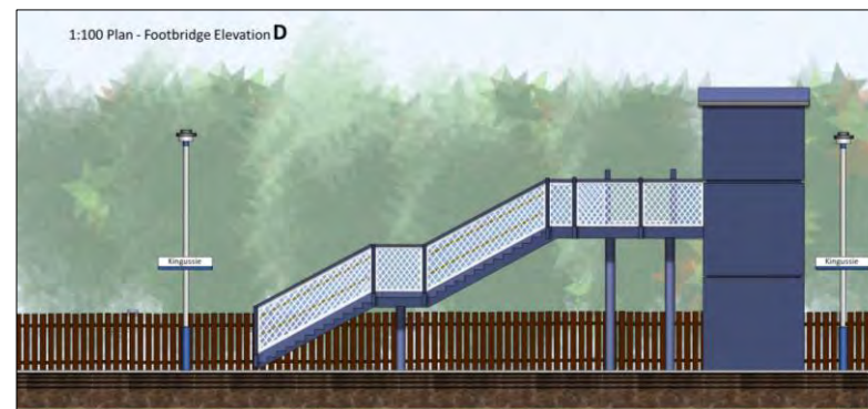
KINGUSSIE STATION ACCESSIBLE FOOTBRIDGE SITE PLAN AND ELEVATION DRAWINGS SCALE 1:100 measurements in metres.
