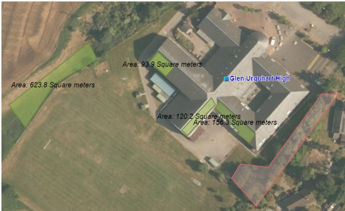
Figure 24: Possible PV Locations
